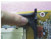
5. Insert the white pushpins onto the black fasteners and press them down firmly to secure the RM on the board.
