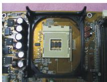
4. Gently press down the black fasteners into the holes until they snap into place.
