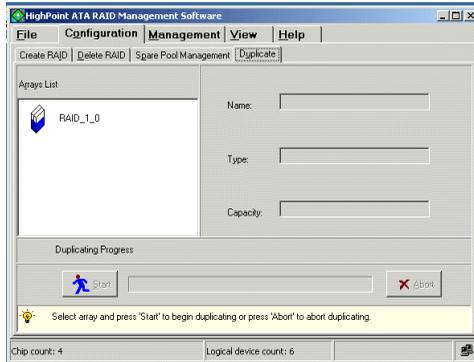
When a RAID 1 or 0+1 array is in critical status, the user can manually duplicate that RAID 1 or 0+1 array.
