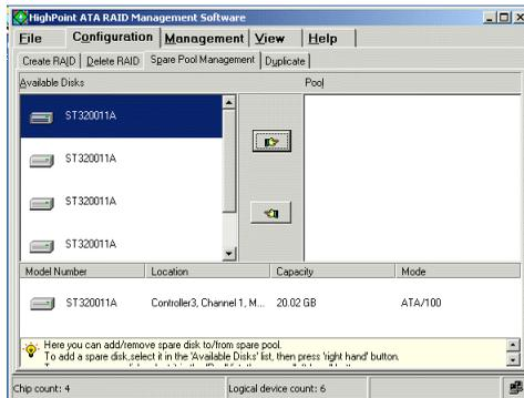
When a disk fails in a mirror array, a spare disk will automatically act as a replacement for the failed disk, and then a rebuilding task will be performed.
